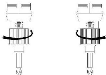
After each adjustment, it is possible to lock the nut with the clutch cover (sold separately). To place properly this cover, you must remove the stopper ring #2, unscrew the adjusting nut #3, unscrew and remove the front ring #1 and replace it with the clutch cover #35 (#37 in KBL30 models).
