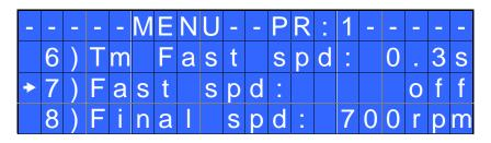
**7)** Fast spd (Fast Speed): It indicates how long the screwdriver should turn at the FAST SPEED speed (see point 8) before switching to "pre-set speed" (lower speed). The "pre-set speed" is the speed set at point 6. This FAST SPEED time can be set from 0.3 to 10.0 sec.
