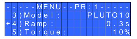
**3) Model:** you can select the screwdriver to be used. Your choice will automatically change the default settings. It's important to select the correct model you're going to use since most parameters regarding the motor software are specific to every single model.
