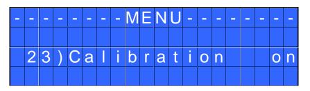
3. Press OK to confirm. If you choose OFF, calibration will be interrupted and no torque value will be displayed. You choose ON, calibration will continue and the following screen will be displayed:
